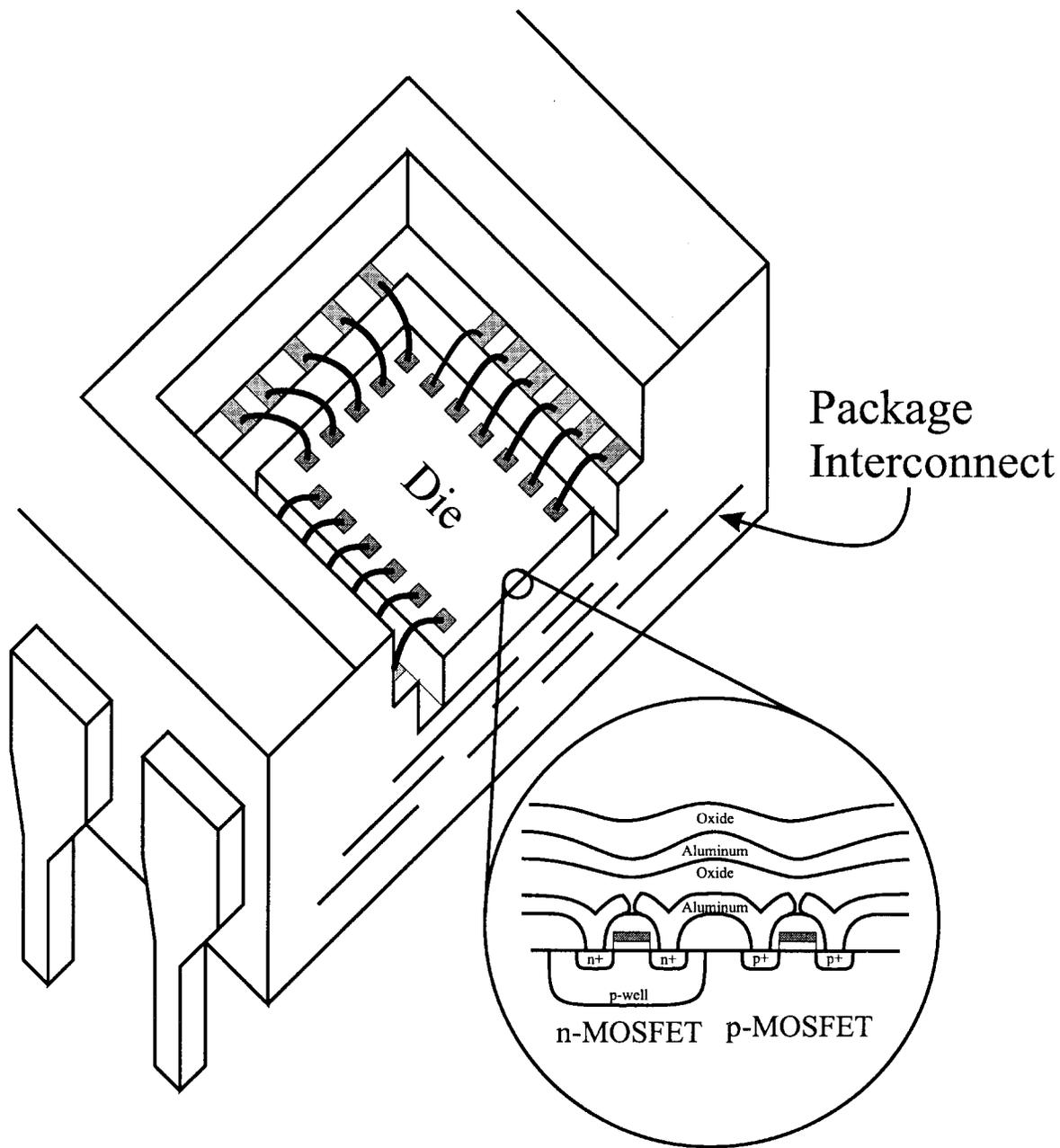
Fig. 9. Typical IC package.
