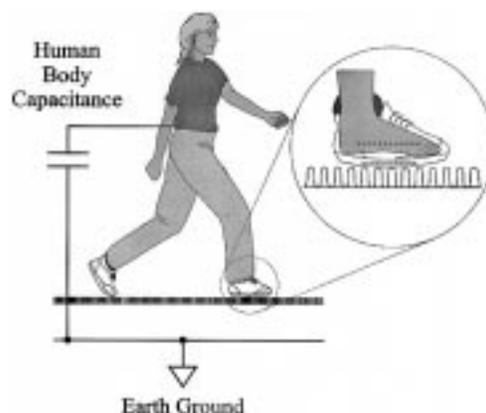
Fig. 2. Triboelectrification illustration.
