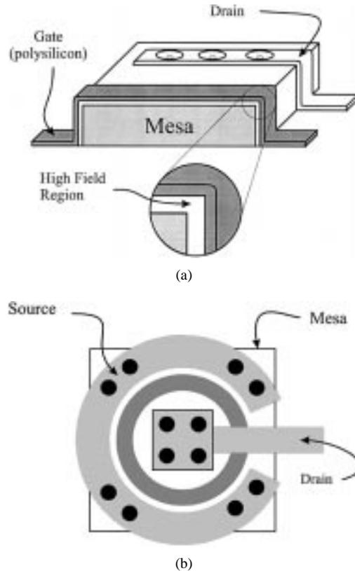
**Fig. 14.** Electric field optimization for ESD protection element. (a) Poor design. (b) Good design.
