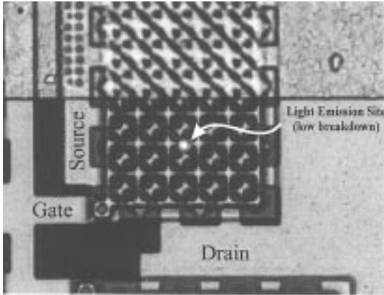
Fig. 15. EMMI photograph showing defect site causing lower breakdown of junction.
