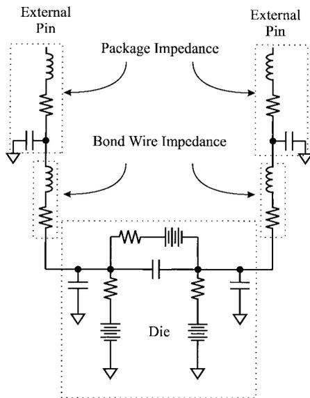
Fig. 10. Package equivalent circuit as seen by an ESD event.
