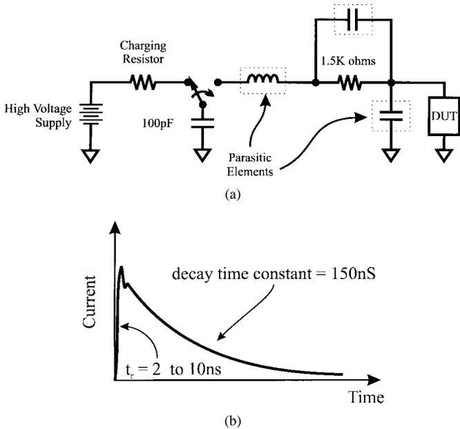
**Fig. 6.** HBM ESD with parasitics. (a) Schematic. (b) Current waveform.
