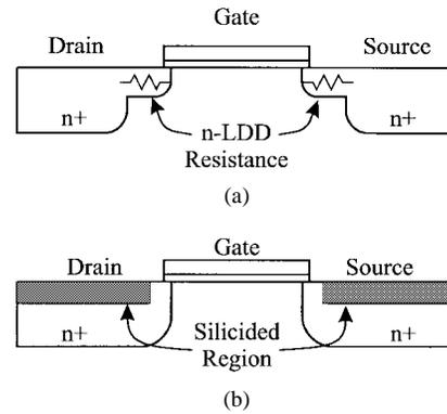
Fig. 17. Advanced process techniques that degrade ESD tolerance. (a) LDD structure. (b) Silicided junction.
