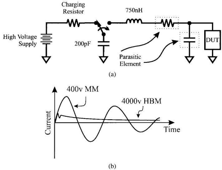
**Fig. 7.** MM ESD with parasitics. (a) Schematic. (b) Current waveform.
