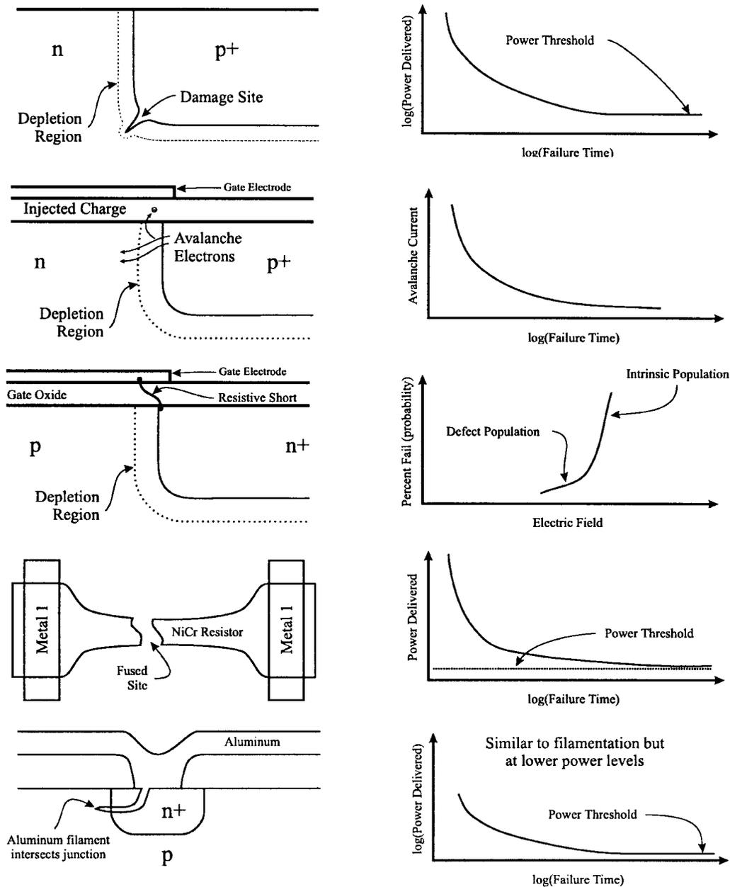
Fig. 18. Damage mechanisms: schematic and failure model.
