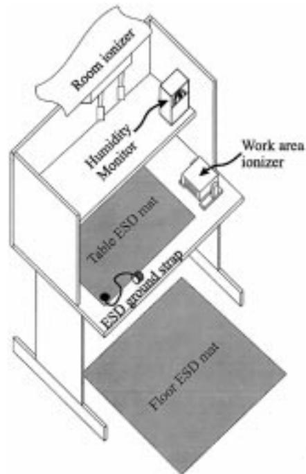
Fig. 5. ESD controls used in an electronics laboratory.
