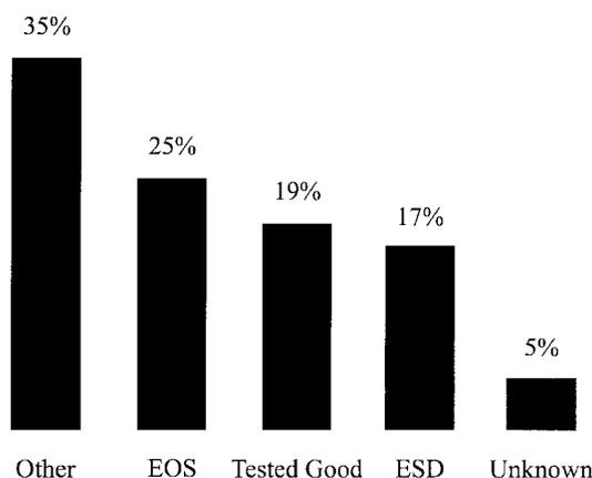
Fig. 1. Field return failure causes.
