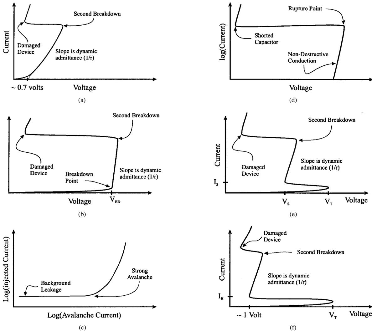
Fig. 12. Nonlinear conduction mechanisms' I-V characteristics. (a) Forward conduction. (b) Junction breakdown. (c) Charge injection. (d) Dielectric breakdown. (e) Snap-back. (f) SCR.
