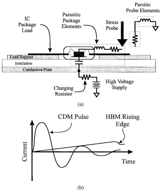
Fig. 8. CDM ESD with parasitics. (a) Schematic. (b) Current waveform.
