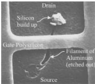
Fig. 16. Resulting short site when the transistor was subjected to EOS.
