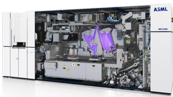
ASML makes machines that our customers use to pattern these small structures on the chip. This is happening at the edges of what physics allows us while it also has to be economically viable. The list of things is very long that we have to control to pattern reliably 200 wafers per hour with 1nm node structures.
