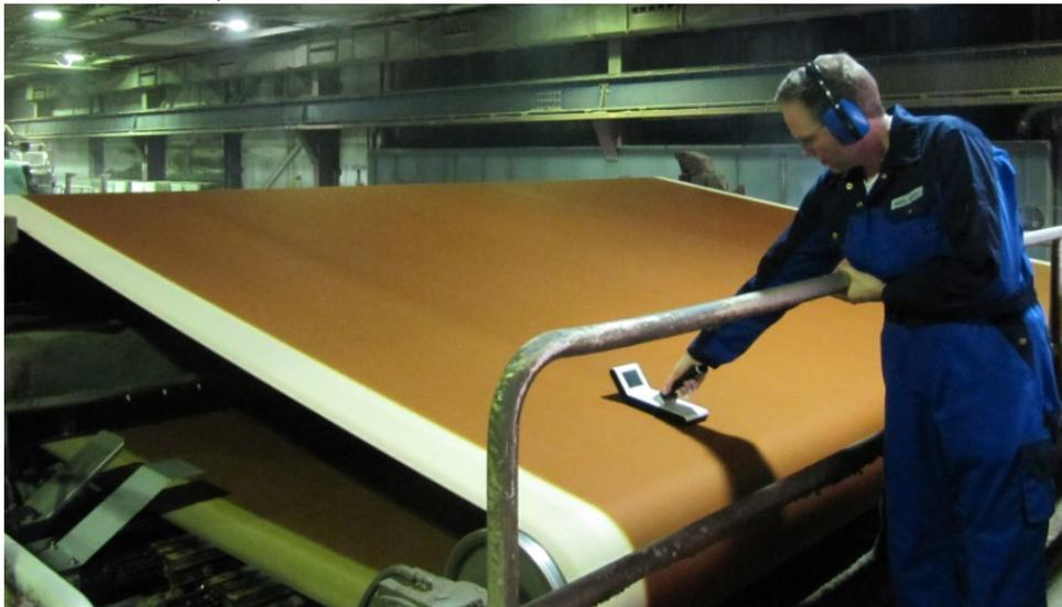
*Above, an impression of a running belt in a paper making machine. On this picture Marcel Lensvelt (owner of Feltest) is holding a prototype of the Aequo moisture sensor, from the 2014 PwI project. The to be developed sensor will likewise be held by hand, either touching or not touching the belt surface. In the picture Marcel is standing behind the moving belt, which is potentially unsafe (if the 400 kg heavy belt would rip with 40 m/s he would get seriously hurt).*
