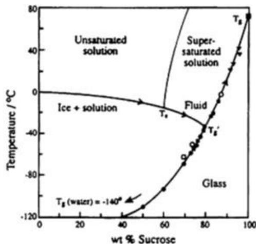
Figure 2 State diagram of a sucrose/water system. Figure taken from F. Franks, *Eur. J. Pharm. Biopharm* 24 221 (1998)
